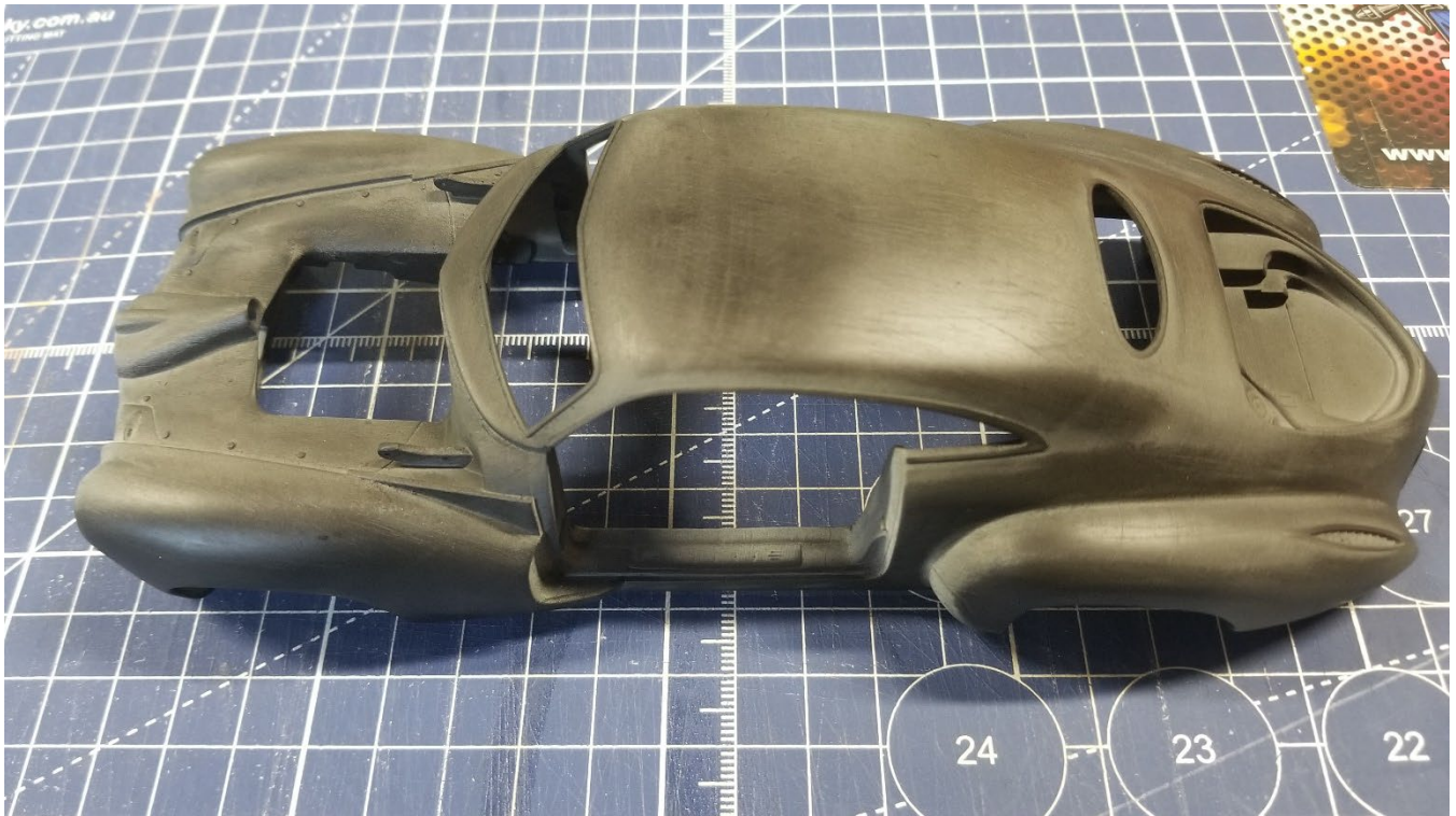
Primer and contrasting colour "blocking" coat applied
